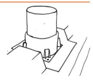
5. Infill ends of profile as shutter for concrete (contractor choice of material – foam/mineral wool etc) Trim if necessary ensuring minimum cover of 75mm around base of QuelCast.
